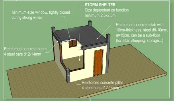
Foundation beam at the top of walls should have the same height reinforcement: four steel bars Φ10–12 mm, steel wire Φ6 mm, 15 cm spacing.
